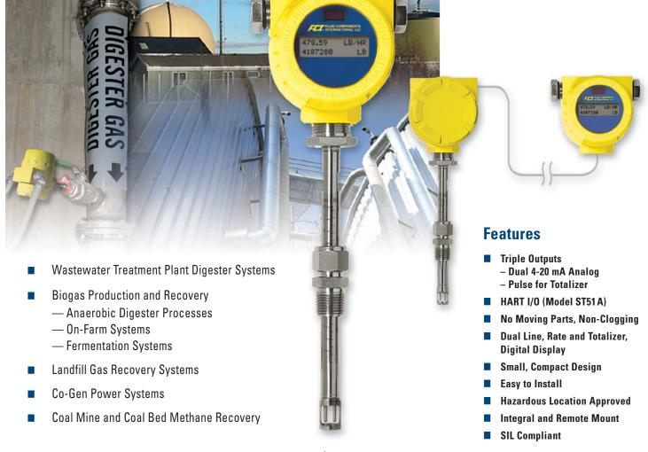
The ST51 Series Flow Meter is an accurate, easy to install, no moving parts solution for measuring and controlling biogases, digester gases, methane and natural gas flow. ST51 utilizes FCI proven thermal dispersion technology to provide direct mass flow measurement resulting in higher performance at a lower cost than orifice plates, DP, Vortex shedding and other thermal devices.
