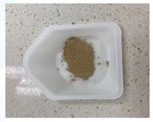
Figure 1. Scale sample from West Africa offshore well.
